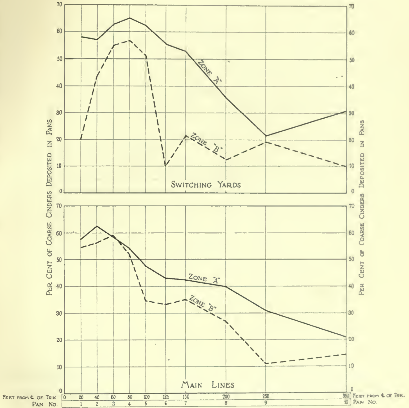
FIG. 715. AVERAGE AMOUNT OF COARSE CINDERS DEPOSITED IN EACH PAN IN PER CENT OF THE TOTAL MATERIALS DEPOSITED IN THE PAN IN QUESTION
